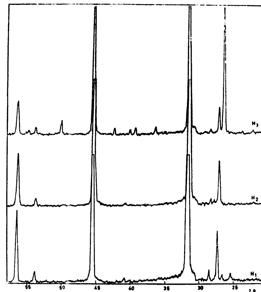
Fig. (1) X-ray diffraction patterns of salt samples H 1 , H 2 , & H 3 .
