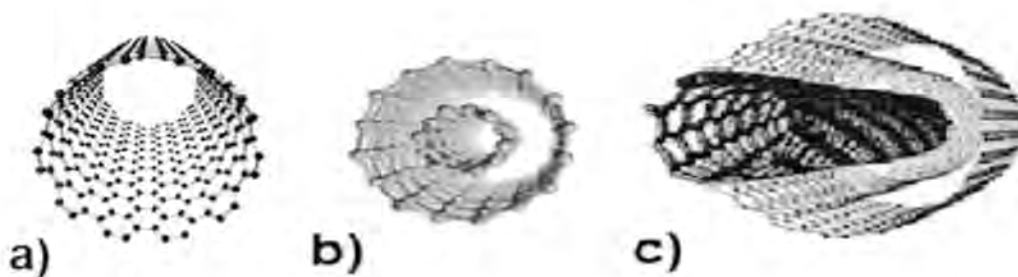
Fig. -1: Schematic of: (a) SWCNT, (b) DWCNT, and (c) MWCNT [1,5]
