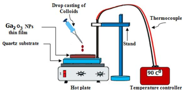
**Figure 2.** Drop casting method to produce cactus-like  $\beta$ -Ga<sub>2</sub>O<sub>3</sub> nanostructures thin film on a quartz substrate at 90°C.
