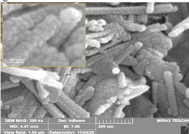
**Figure 6.** The SEM images of cactus-like  $\beta$ -Ga<sub>2</sub>O<sub>3</sub> nanostructure thin films prepared at laser fluency (5.57J/cm<sup>2</sup>).
