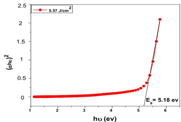
**Figure 8.** The energy gap of cactus-like  $\beta$ -Ga<sub>2</sub>O<sub>3</sub> nanostructure thin films at laser fluency 5.57 J/cm<sup>2</sup>..
