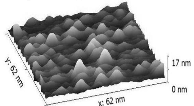
**Figure 4.** The AFM images of cactus-like  $\beta$ -Ga<sub>2</sub>O<sub>3</sub> nanostructure thin films prepared at laser fluency (5.57J/cm<sup>2</sup>).
