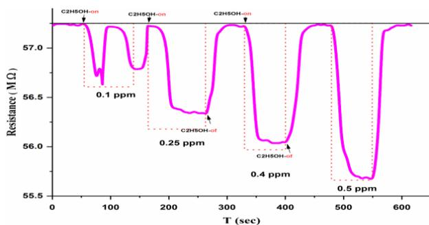
**Figure 9.** The response of cactus-like  $\beta\text{-Ga}_2\text{O}_3$  nanostructure sensor to different concentrations of ethanol gas at laser fluency  $5.57 \text{ J/cm}^2$ .
