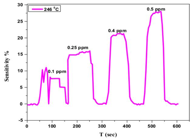
**Figure 10** The sensitivity of the cactus-like  $\beta\text{-Ga}_2\text{O}_3$  nanostructure thin films sensor to ethanol ranging from 0.1 to 0.5 ppm for 10 min.
