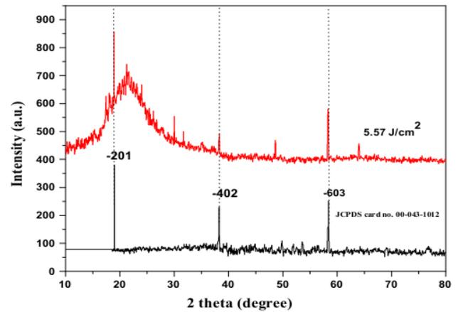
**Figure 3.** X-ray diffraction patterns of cactus-like  $\beta$ -Ga<sub>2</sub>O<sub>3</sub> nanostructure thin films at the laser fluency 5.57 J/cm<sup>2</sup>
