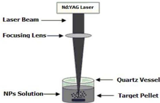
**Figure 1.** PLAL technique to produce a spindle-like  $\beta$ -Ga<sub>2</sub>O<sub>3</sub> nanostructures.
