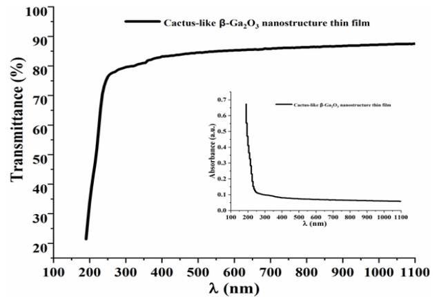
**Figure 7.** UV-vis transmittance and absorbance spectra of cactus-like  $\beta$ -Ga<sub>2</sub>O<sub>3</sub> nanostructure thin films at laser fluency 5.57J/cm<sup>2</sup>.
