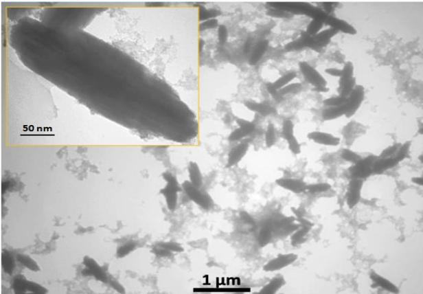
**Figure 5.** The TEM images of spindle-like  $\beta$ -Ga<sub>2</sub>O<sub>3</sub> nanostructure colloids at laser fluency (5.57 J/cm<sup>2</sup>).
