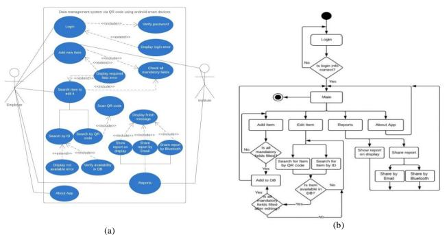
Figure 1. (a) Use Case Diagram; (b) Activity Diagram
