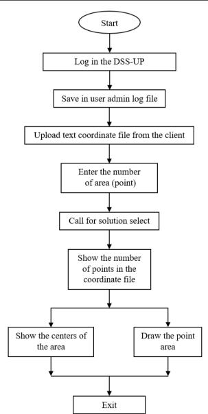
Figure 1. Process the system flow of DSS-up platform.
