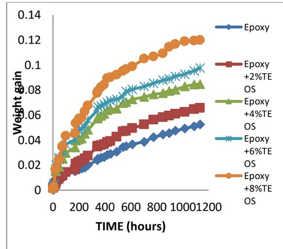
Figure 2: Water absorption as a function of time
