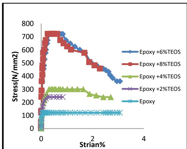
Figure 4: Stress- strain curve after immersion water
