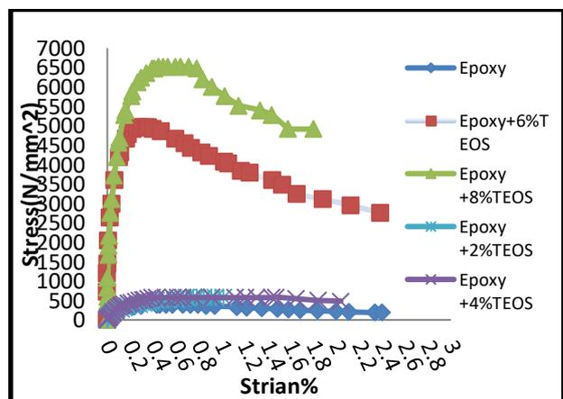
Figure 3: Stress-strain curve before immersion water
