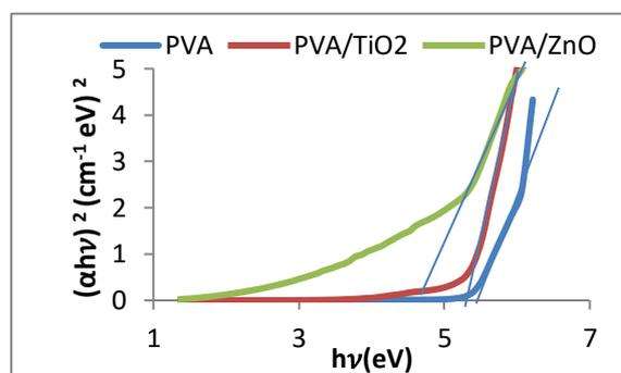
Figure 5: Plot of  $(\alpha h\nu)^{1/p}$  against photon energy of (PVA) polymer, PVA/ TiO<sub>2</sub> and PVA/ ZnO polymer solutions.
