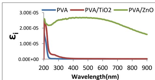
Fig. 10: imaginary part of dielectric constant with wavelength of (PVA) polymer, PVA/ TiO<sub>2</sub> and PVA/ ZnO polymer solutions.
