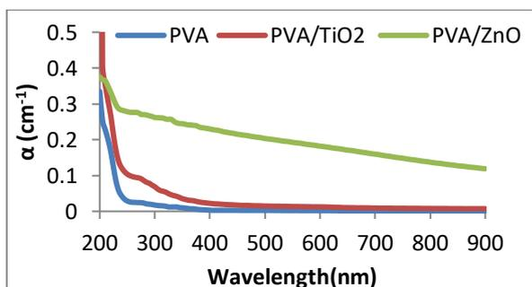
Figure 4: Optical absorption coefficient  $\alpha$  as wavelength of (PVA) polymer, PVA/ TiO<sub>2</sub> and PVA/ ZnO polymer solutions.
