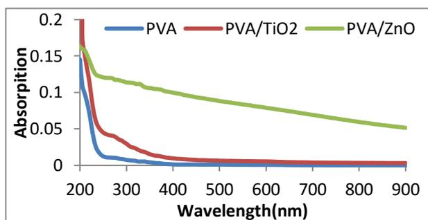
Figure 3: Optical Absorption spectra of (PVA) polymer, PVA/ TiO<sub>2</sub> and PVA/ ZnO polymer solutions.
