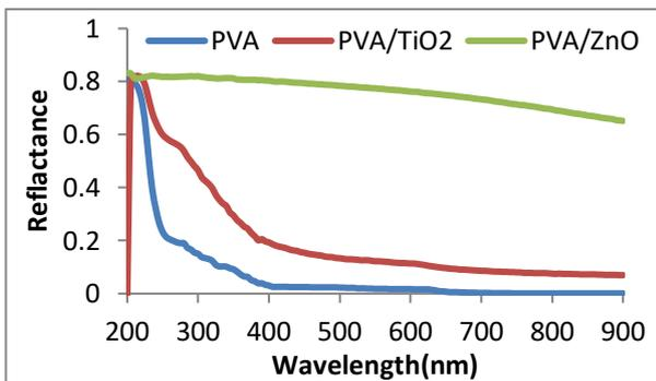
Figure 6: Optical Reflectance as wavelength of (PVA) polymer, PVA/ TiO<sub>2</sub> and PVA/ ZnO polymer solutions.
