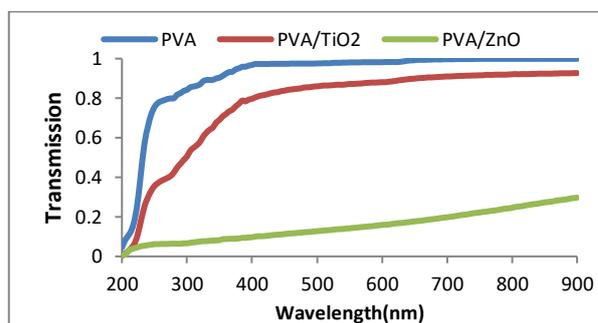
Figure 2: Optical Transmittance of (PVA) polymer, PVA/ TiO<sub>2</sub> and PVA/ ZnO polymer solutions.
