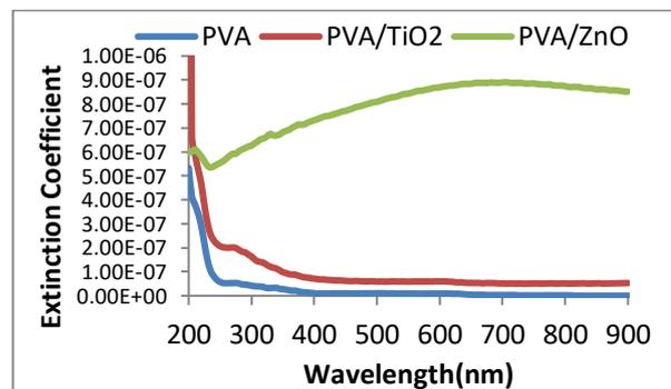
Figure 8: Dispersion of extinction coefficient (k) with wavelength of (PVA) polymer, PVA/ TiO<sub>2</sub> and PVA/ ZnO polymer solutions.
