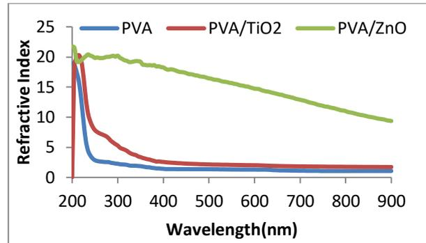
Figure 7: Dispersion of refractive index (n) of (PVA) polymer, PVA/ TiO<sub>2</sub> and PVA/ ZnO polymer solutions.
