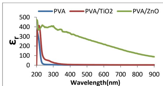
Figure 9: Real part of dielectric constant with wavelength of (PVA) polymer, PVA/ TiO<sub>2</sub> and PVA/ ZnO polymer solutions.
