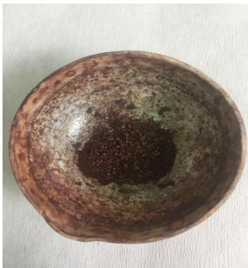
Figure 5- nanoparticles produced after being placed in the oven under 400 degrees heating
