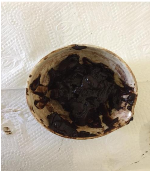
Figure 4- The nanoparticles produced before being placed in the oven to be transformed into a small nanoparticle by heating 400 degrees
