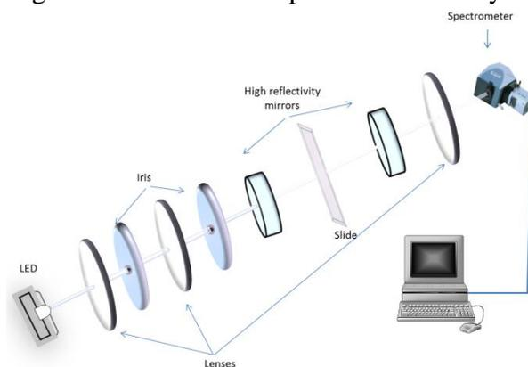
**Figure (2):** The setup of Broadband Cavity Enhanced Absorption Spectroscopy for the thin film.
