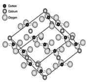
Figure 1: The crystal structure of calcite.
