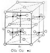
Figure 2: The crystal structure of aragonite.
