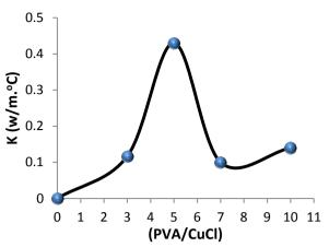
Figure 1: Thermal conductivity of (PVA-CuCl) at frequency 100(Hz).
