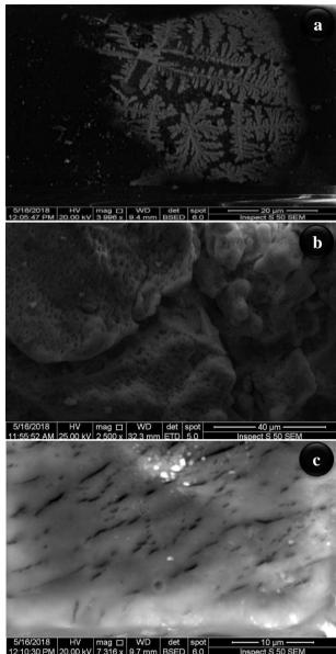
Figure 4: SEM Image (a) CuCl Powder, (b) 5% PVA/ CuCl, (c) 7% PVA\_CuCl.
