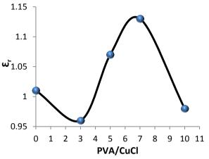
Figure 2: Dielectric Constant of (PVA -CuCl) at frequency 100(Hz).
