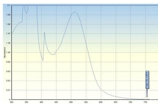
Figure 2: Absorption spectra of 50  $\mu\text{g}/\text{ml}$  of CFD-2,5-DMP against the reagent blank at 510 nm.
