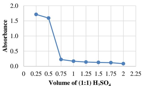
Figure 3: Effect of (1:1) H<sub>2</sub>SO<sub>4</sub> volume.
