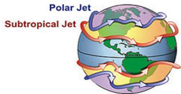
Figure 2. The polar and subtropical jet streams [5].
