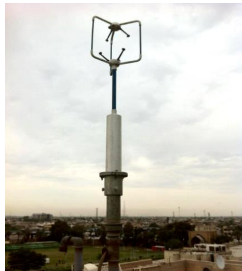
Figure 1: Ultrasonic anemometer device above the building Al-Mustansiriyah University College of sciences.
