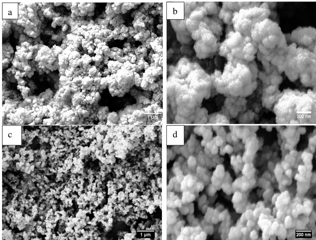
**Figure 4.** FESEM photo of (a,b) pure SiO<sub>2</sub> (NPs), (c,d) SiO<sub>2</sub> with silicon sealant.
