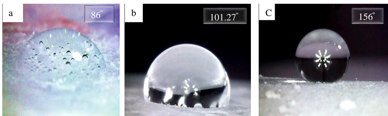
**Figure 6.** water contact angle of (a) pure SiO<sub>2</sub> (NPs), (b) pure silicon sealant elastomers. (c) superhydrophobic surface on glass .
