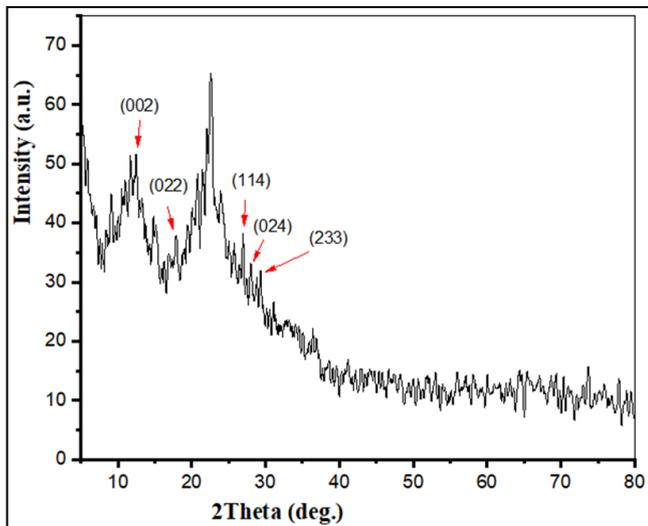
**Figure 3.** XRD pattern of SiO<sub>2</sub>(NPs) synthesis by sol-gel method.
