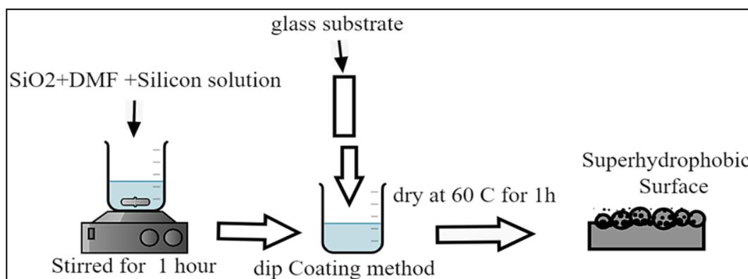
**Figure 2.** scheme diagram for the synthesis of superhydrophobic surfaces.
