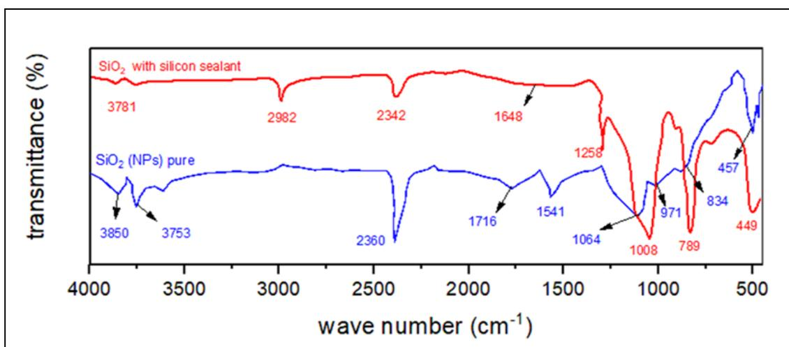
Figure 5. FTIR of pure ( SiO<sub>2</sub> ) and SiO<sub>2</sub> modified with silicon sealant.
