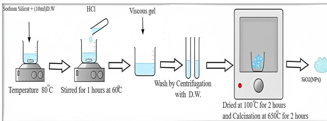
**Figure 1.** Schematic digram for the preparation of SiO<sub>2</sub> (NPs) by Sol-gel method.
