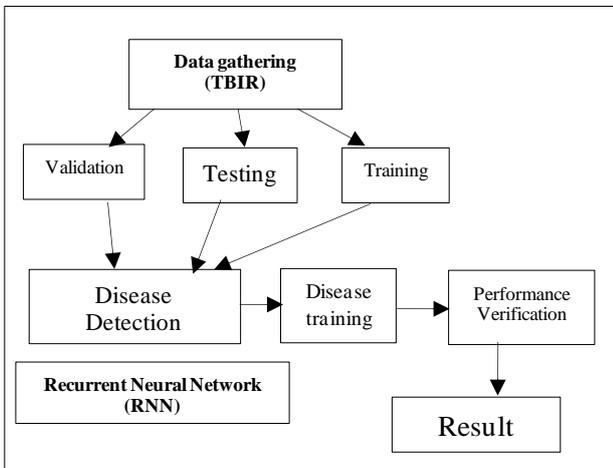
Figure 3. Flow chart of Texture Based Image Retrieval.
