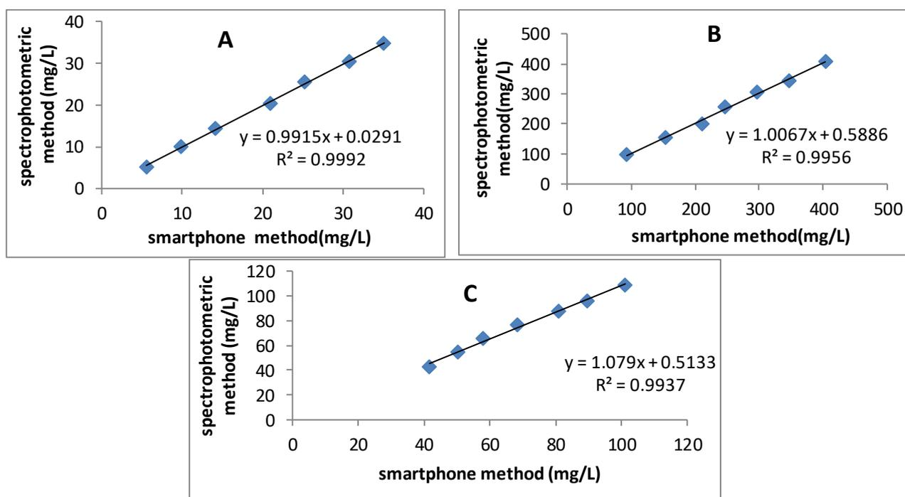
Figure 8: Correlation curves of A- M.B dye, B- M.R dye and C- M.O dye concentrations obtained with the smartphone method and the classical method.
