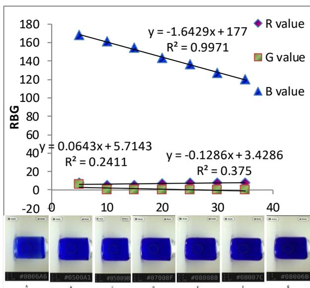
Figure 2: Calibration curve and linearity equations for determination of M.B standard solutions. The inset shows the screenshots for M.B standard solutions using Colormeter App. programs.
