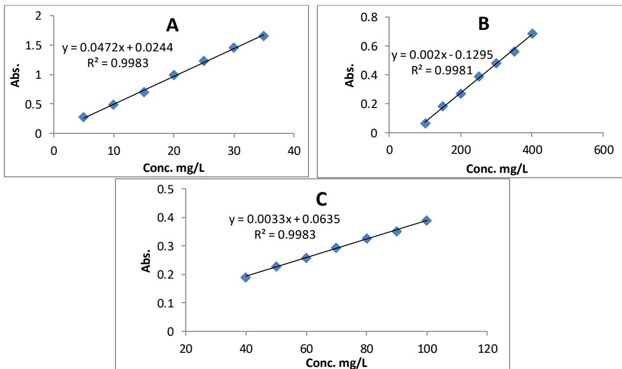
Figure 7: Calibration curves: (A) for M.B at concentrations (5-35 mg/L) (B) for M.R at concentrations (100-400 mg/L) (C) for M.O at concentrations (40-100mg/L)
