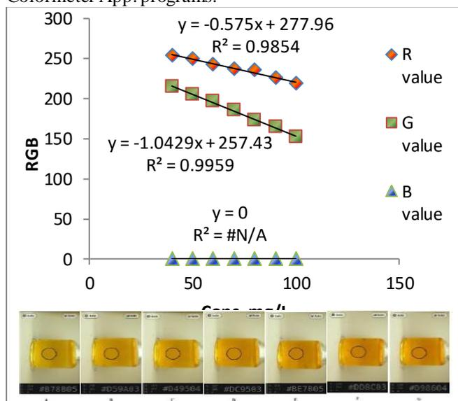
Figure 4: Calibration curve and linearity equations for determination of M.O standard solutions. The inset shows the screenshots for M.O standard solutions using Colormeter App. programs.
