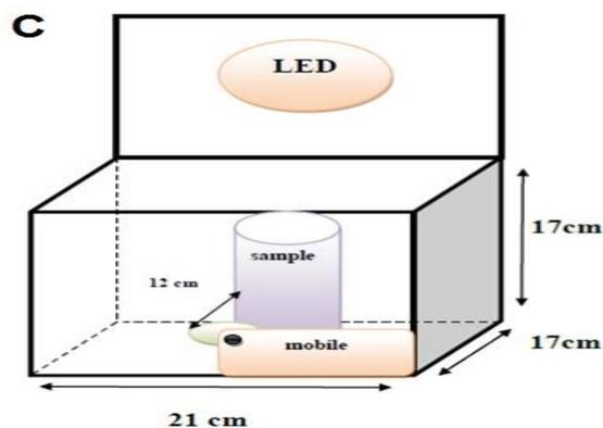
Figure 1: Colorimetry instrument of smartphone digital image; (a) a photo of smartphone colorimetry instrument with an open cover and M.R dye as a sample, (b) a photo of a smartphone colorimetry instrument with a closed cover and M.O dye as a sample and (c) Schematic diagram.
