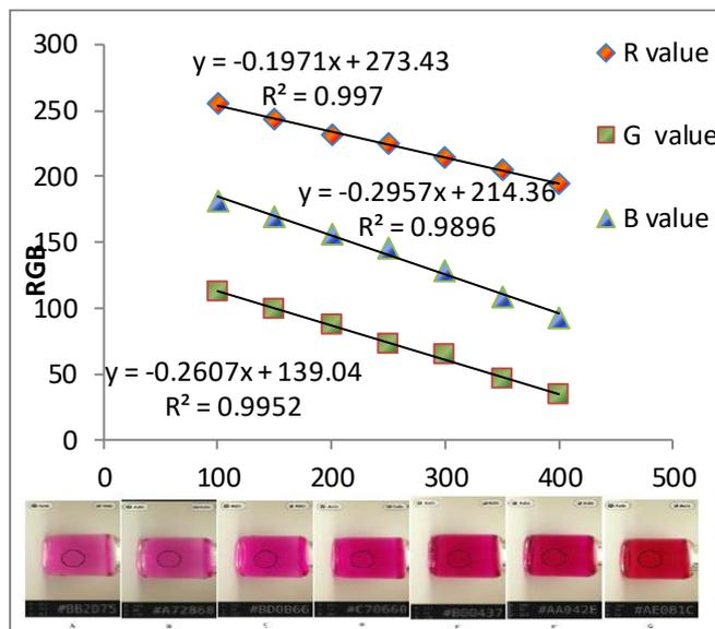
Figure 3: Calibration curve and linearity equations for determination of M.R standard solutions. The inset shows the screenshots for M.R standard solutions using Colormeter App. programs.
