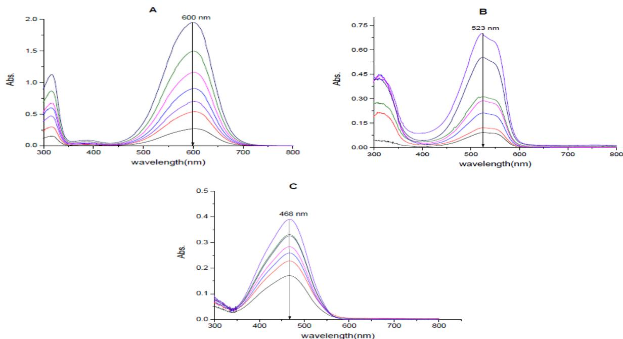
Figure 6: Absorption spectrum (A) for M.B at concentrations (5-35 mg/L) (B) for M.R at concentrations (100-400 mg/L) (C) for M.O at concentrations (40-100mg/L)
