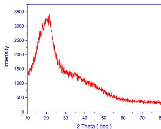
Figure 1. XRD pattern of activated carbon.
