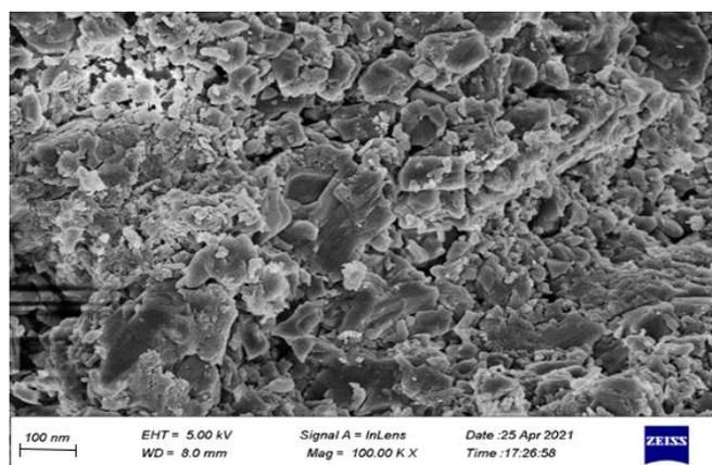
Figure 2. SEM image of activated carbon Nanoparticles.
