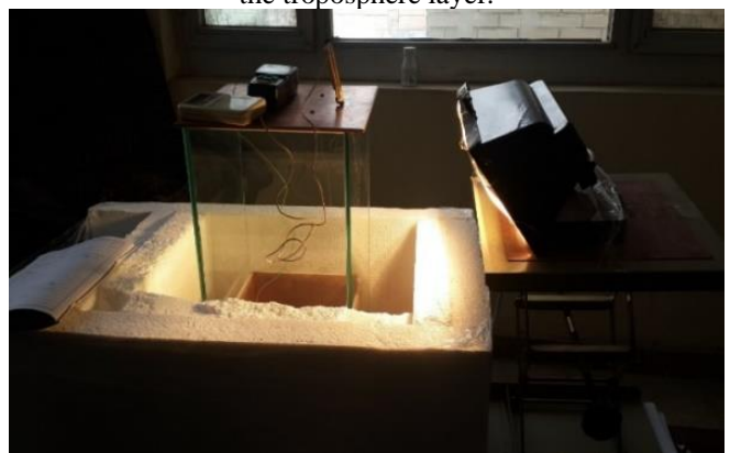
Figure 8. The designed cloud chamber during the test.
