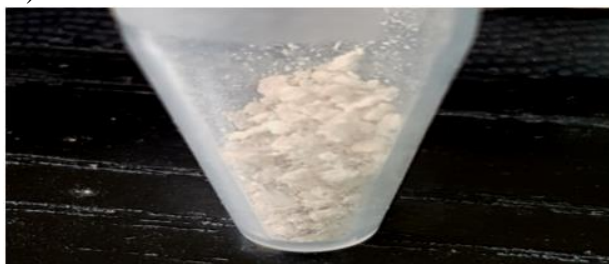
Figure 5: PHA polymer after extraction and drying Polymer analysis by FTIR.
