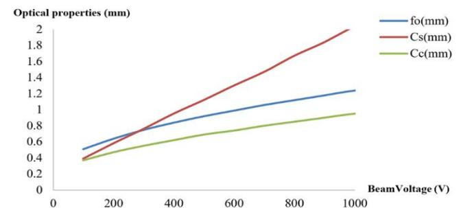
Figure 7. Comparison of optical properties as a function of beam voltage and at constant values for inner bore diameter 55mm.
