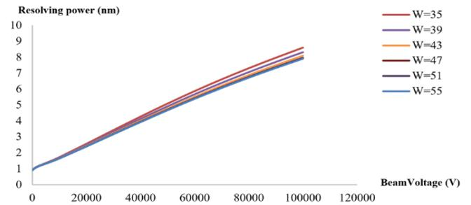
**Figure 12.** Comparison of resolving power curves as a function of beam voltage.
