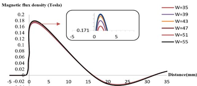
Figure 3. The distribution of axial magnetic flux density ( $B_z$ ) as a function of the distance ( $Z$ ) of the designed lenses.
