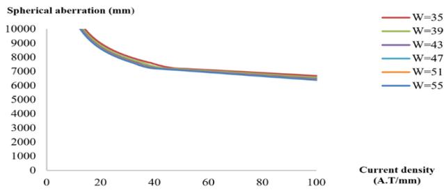
**Figure 9.** Comparison of spherical aberration curves as a function of current density.
