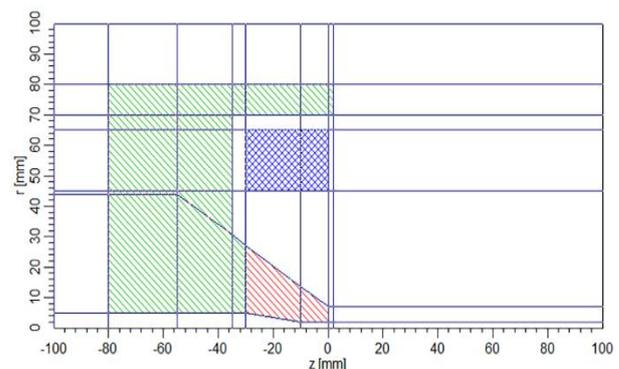
Figure 1. Cross-section of a magnetic unipolar lens prototype [19].
