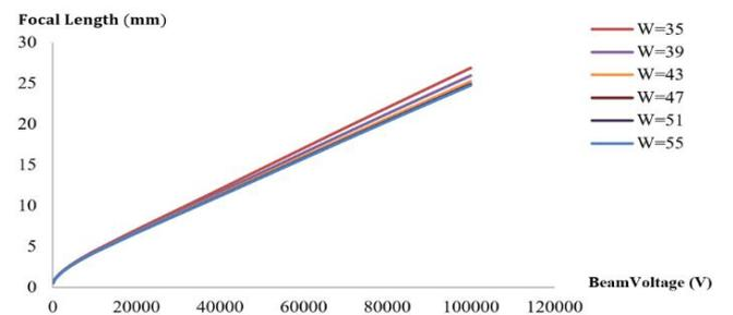
Figure 6. Comparison of focal length curves as a function of beam voltage.
