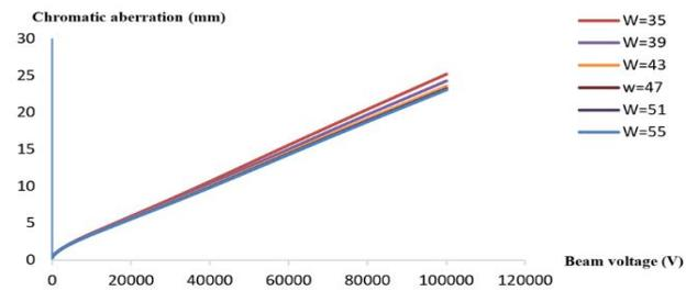
Figure 4. Comparison of chromatic aberration curves as a function of beam voltage.
