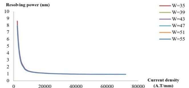
**Figure 13.** Comparison of resolving power curves as a function of current density.
