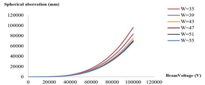
Figure 5. Comparison of spherical aberration curves as a function of beam voltage.
