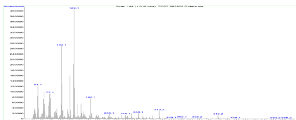
Figure 5. The electrospray (+) mass spectrum of [\text{Co}(\text{L})(\text{H}_2\text{O})\text{Cl}_2] .
