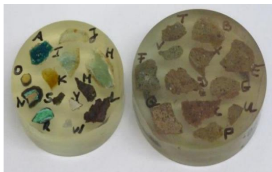
Figure 2. Left: Glass and metal samples embedded in epoxy resin. Right: Ceramic samples embedded in epoxy resin.
