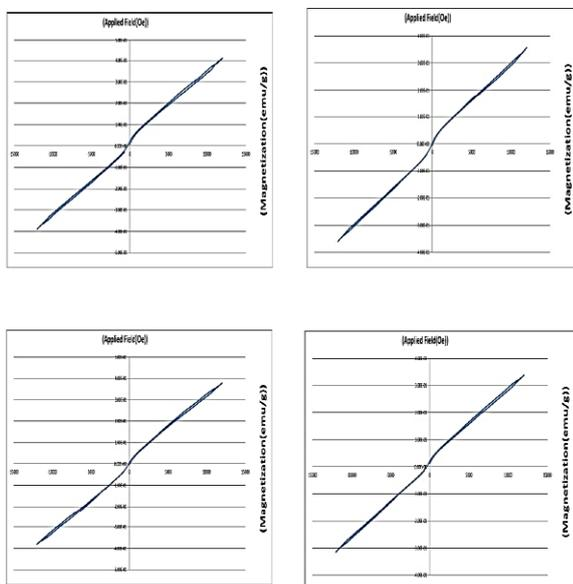
**Figure 4.** magnetization versus magnetic field M-H for Bi PbSrCaCuZn<sub>x</sub>O at variable concentration Zn (x= 0.2, 0.4, 0.6, 0.8, and 1).
