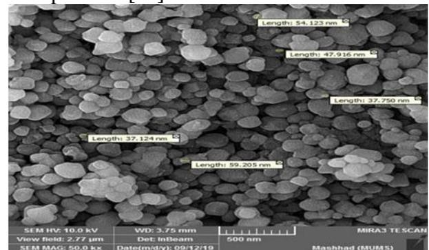
**Figure 4.** FESEM image of TiO<sub>2</sub> nanoparticles biosynthesized by *Lactococcus lactis* ssp. *lactis*.
