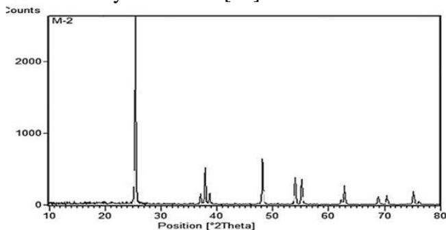
**Figure 3.** XRD pattern of TiO<sub>2</sub> nanoparticles biosynthesized by *Lactococcus lactis* ssp. *lactis*.
