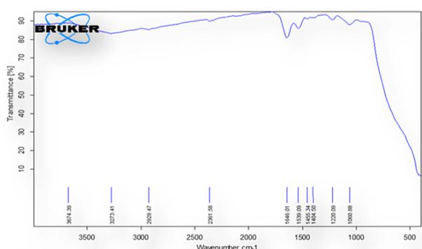
**Figure 6.** FTIR results of biosynthesized TiO<sub>2</sub> nanoparticles by *Lactococcus lactis* ssp. *Lactis*.
