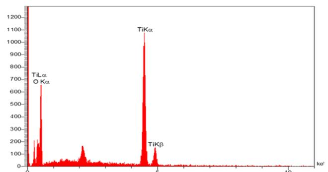
**Figure 5.** EDX of biosynthesized TiO<sub>2</sub> nanoparticles by *Lactococcus lactis* ssp. *lactis*.
