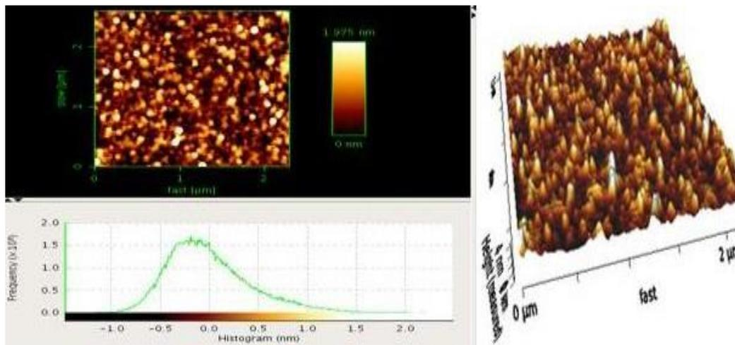
**Figure 2.** AFM of TiO<sub>2</sub> nanoparticles biosynthesized by *Lactococcus lactis* ssp. *lactis*.
