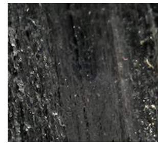
Digital microscopy for ER6010 alloy + SnS under load 13 kg.
