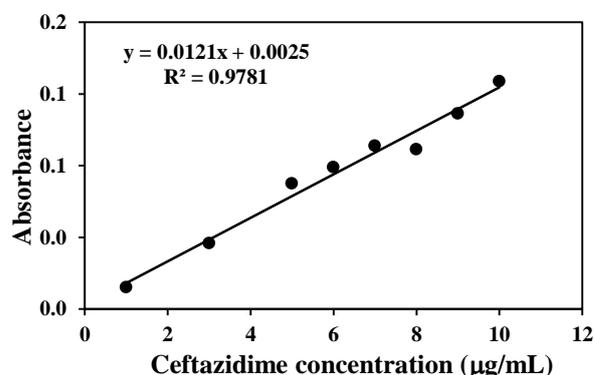
Figure 9: Standard calibration curve of Ceftazidime.
