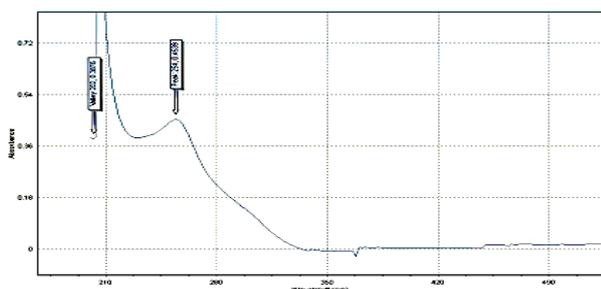
**Figure 2:** The absorption spectrum of 10 µg/mL of a standard solution of ceftazidime vs solvent blank.
