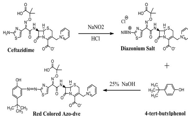
Figure 8: The suggested mechanism of diazotization and coupling reactions [20].
