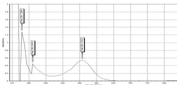
**Figure 3:** The spectrum of 20 µg/mL solution of Ceftazidime-4-tert-butylphenol versus the reagent blank recorded under the optimal conditions.
