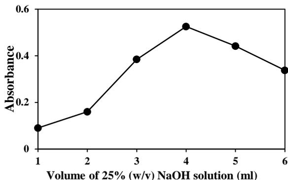
Figure 6: The effect of the volume of the NaOH solution.
